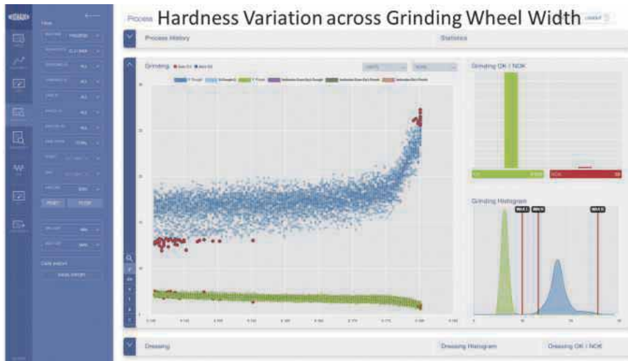
Figure 2: Hardness variation across the threaded grinding wheel width
