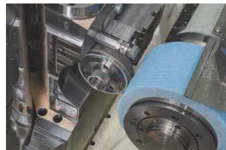
With a 5-pass full profile roll, the dressing time can be reduced by more than half without compromising on quality
