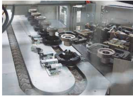
Loading to and unloading from the conveyor belt is done by a transfer unit
