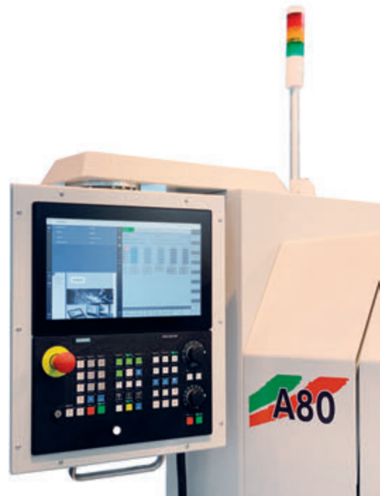
In the CNC used all the software functions, automation included, are integrated into those of the machine through the exclusive HMI software platform belonging to Ghiringhelli
