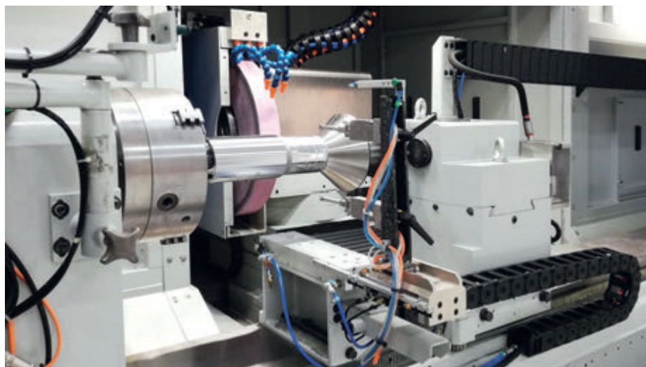
The wheelhead can perform machining for external, internal, shoulder, face, conical, complex profiles and threads grinding
