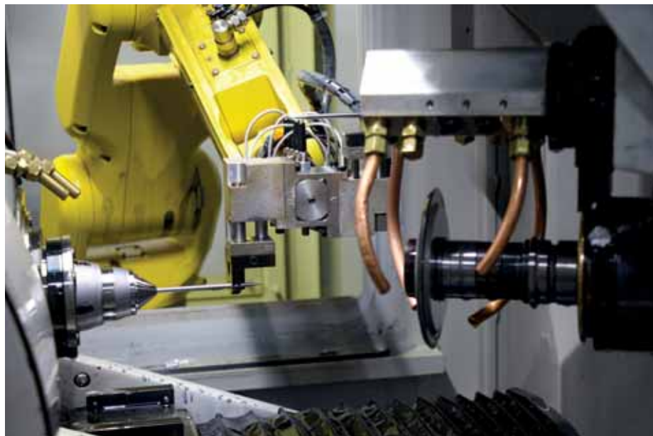
Speedy automation is one reason Tru-Edge makes its medical customers happy. Here, one robot gripper on an ANCA MX7 removes a finished surgical instrument just before its twin swings down to load the next blank
