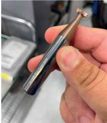
ARCH Cutting Tools delivered this custom engineered, solid carbide keyseat cutter, with coating, in under 48 hours
