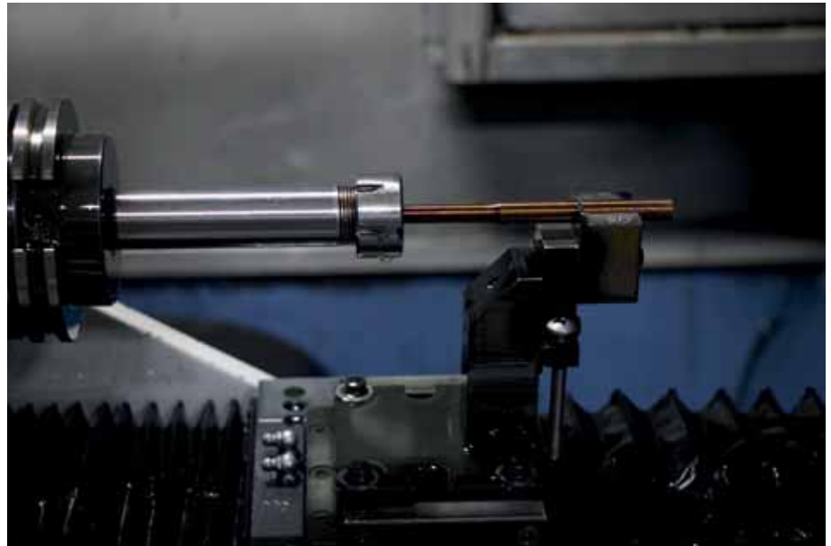
Tru-Edge relies on ANCA's traveling steadyrest and part specific bushings to keep tools perfectly straight during the grind
