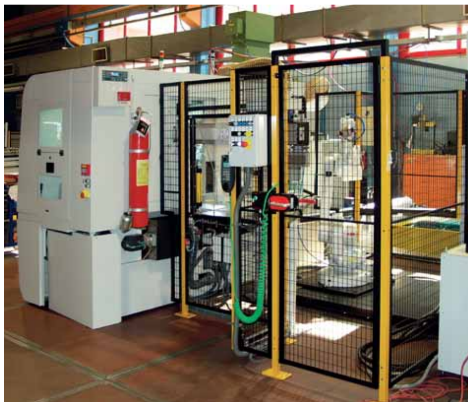
All the software functions, automation with robotic systems included, are combined to those of the machine through the exclusive HMI Ghiringhelli interface
