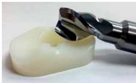
ARCH Cutting Tools produces a unique 3-flute carbide helical cutter that delivers unequalled part finish, higher throughput, and longer tool life in machining a polyethylene tibial insert
