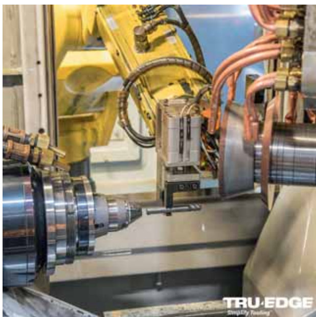
Metalworking tools, like this carbide ball nose endmill, account for most production at Tru-Edge
