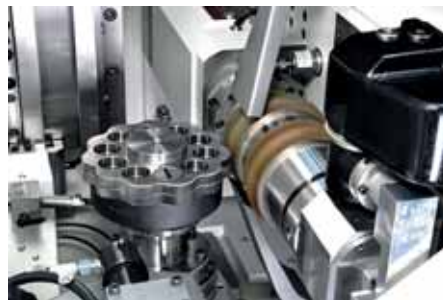
Figure 1: External cycloid machining on the KAPP NILES Gear Centre KX 300 P.
