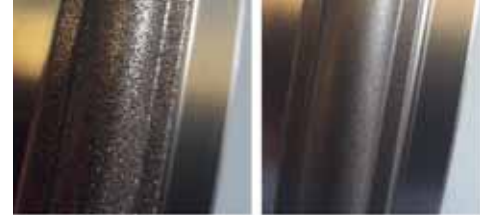
Figure 6: Galvanically bonded CBN wheels in roughing and finishing version.
