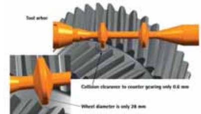
Figure 3: Machining of a double helical cut planetary gear.
