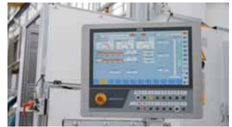
MS-U honing control, latest generation with touch operation panel.
