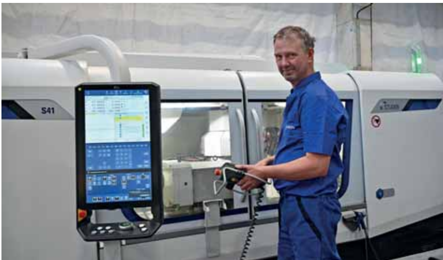
Jaromir Hornych - grinder, on the STUDER CNC universal cylindrical grinding machine S41.
