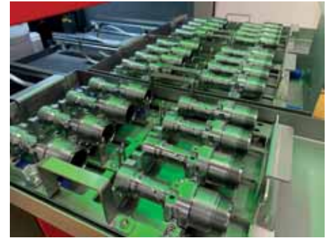
Product carriers with hydraulic blocks that Intercable Tools will be able to deburr automatically in future using ultrasonic deburring technology.
