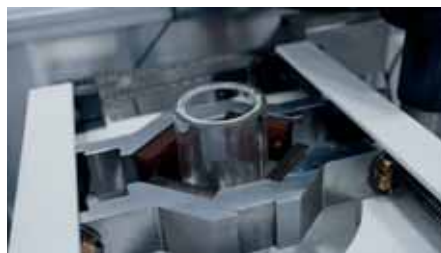
Workpiece centering and clamping, integrated within the honing fixture.
