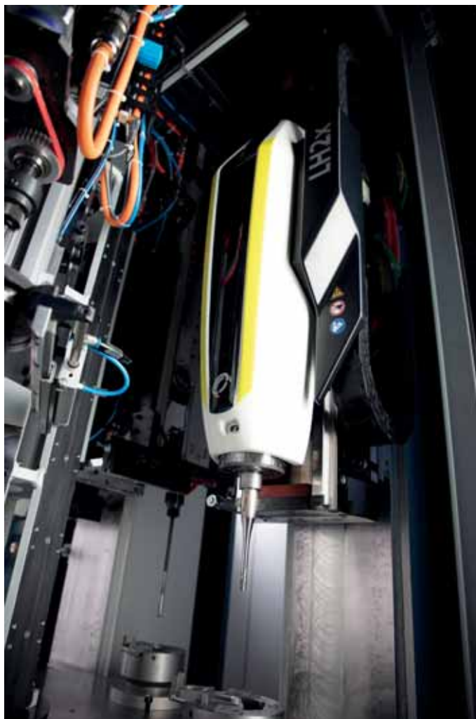
More power, more precision, more potential: The new LH2x honing spindle with three direct drives and four patents is driving the future of honing.
