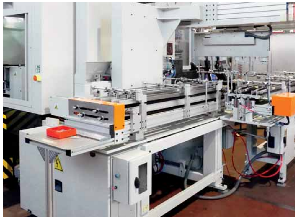
The implemented solution envisaged the implementation of an automatic loading and unloading system designed and manufactured by Ghiringhelli.
