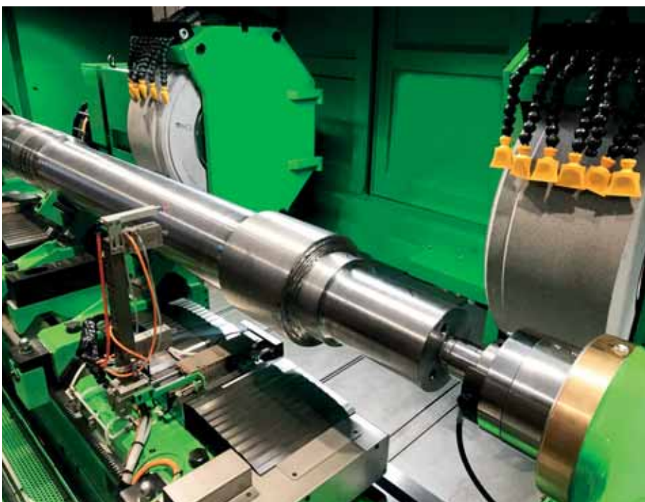
The machine is equipped with a double grinding wheel carriage for simultaneous operations.
