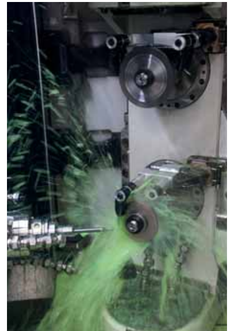
The vertically aligned spindles on the VHybrid with the erosion disc in the lower spindle position.
