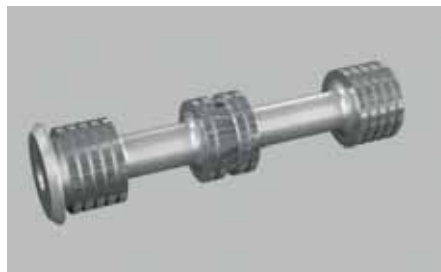
Example image of a control piston - Possible machining task: Face grinding of the control edges on a STUDER S11.
