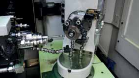
A solid tipped PCD drill being processed on the VOLLMER VHybrid 260.
