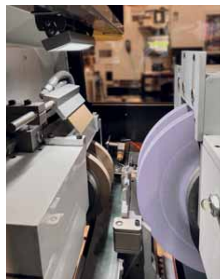
Its highly flexible design allows for rapid reconfiguration of the machine setup to grind fasteners, from one to four pieces simultaneously per grinding cycle.
