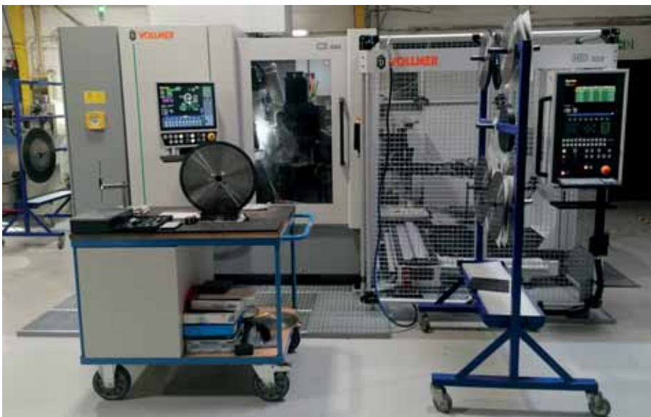
Since the beginning of 2026, Katthöfer Cutting Tools has been using the VOLLMER CS 860 grinding machine together with the ND 320 handling system for the fully automated processing of carbide-tipped circular saw blades.
