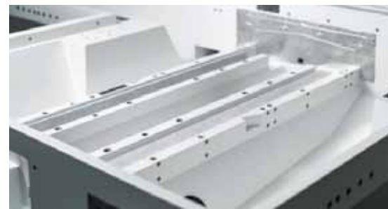
Near-net-shape casting thanks to Granitan technology.
