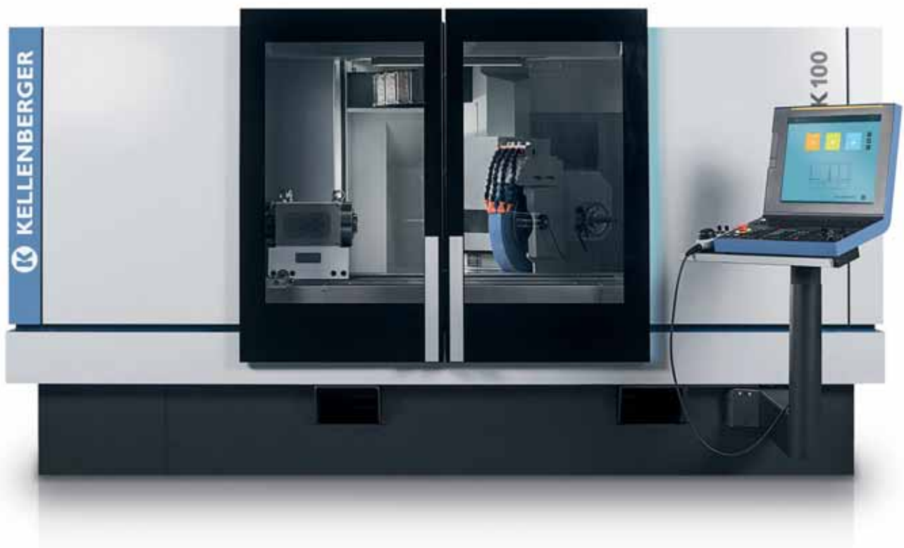
The KELLENBERGER K100 is available in grinding lengths of 600, 1,000 and 1,700 mm.
