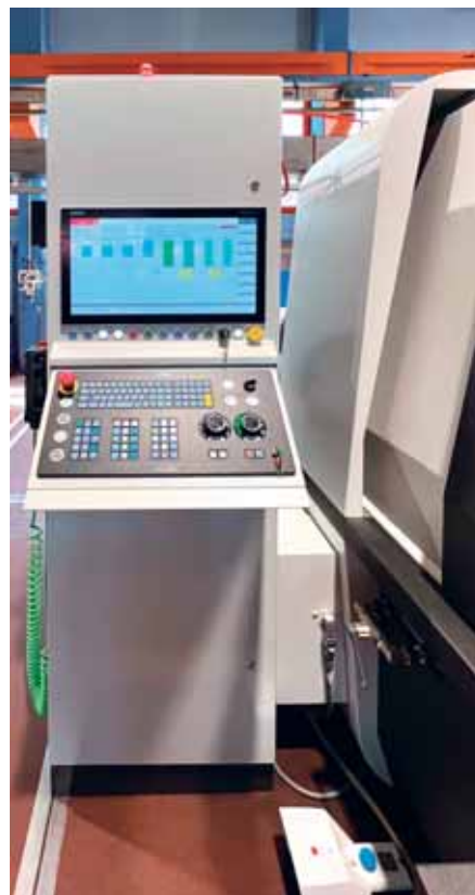
The CNC digital native Siemens Sinumerik-ONE with the "Safety Integrated Plus" module is managed through the HMI interface owned by Ghiringhelli.
