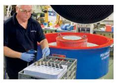
parts machined to extremely tight tolerances are suitable candidates for vibro finishing. As the latter may not be generally appreciated, a number of case studies will be cited where PDJ Vibro equipment is being used to automate the finishing of very high precision components, without surface damage or dimensional change.
