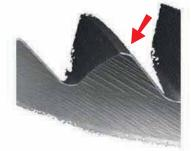
Tap unprocessed (left) and processed (right) in OTEC machines
