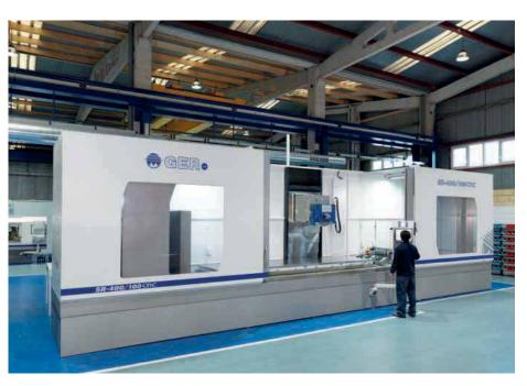
slideways incorporate precision ball screws, FANUC drive motors and Heidenhain linear scale feedback.
