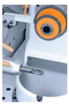
The new optional roughing unit for the Vgrind 360 enables automatic opening of the abrasive coating during production
