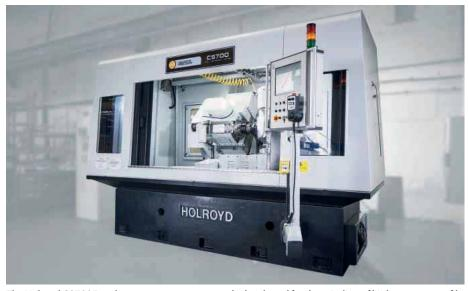
The Holroyd CS700E tool management centre: newly developed for the grinding of high accuracy profile forms on finish milling cutters of up to 700 mm in diameter
