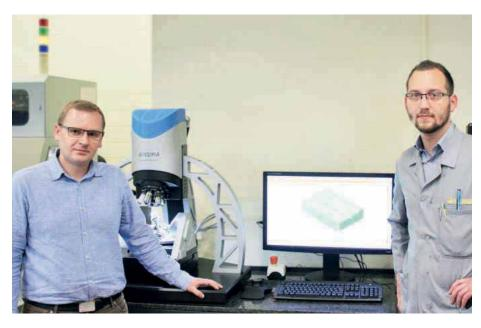
systems for form and roughness measurement of micro-precision dies
