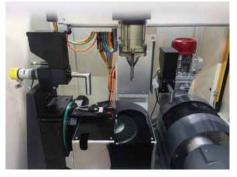
Magnetfinish machine for cutting tools
