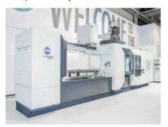
The Multigrind CB XL is designed for the full-sequence machining of large workpieces up to 3,200 mm in length
