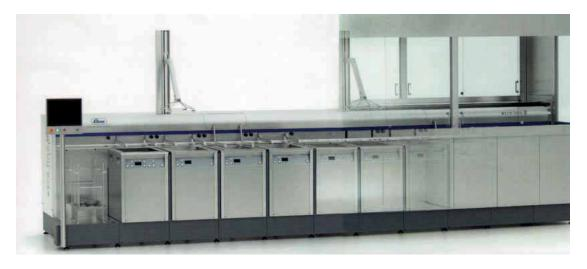
Available in a variety of sizes, they feature a welded stainless-steel tank, double lid with thermal and acoustic insulation, thermostatically controlled indirect heating in the side walls, and an electronic control with digital time/temperature display. A level guard cuts off the heating and ultrasonics if there is insufficient liquid in the tank.
