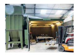
using chilled iron abrasive. Located inside an existing building, the chamber is 6 m long x 4.5 m wide, with walls and roof manufactured from double-skinned insulated steel panels, which reduce sound transmission. The floor is lined with steel plate. Air inlet ducts and exhaust points around the chamber ensure effective dust extraction and air ventilation.
