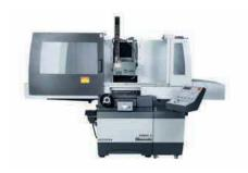
Equally suited to piece part work in a toolroom or prototype area or even small part volume production, standard features of this well specified machine include automatic grinding cycles and intuitive controls to simply machine operation and optimise productivity.
