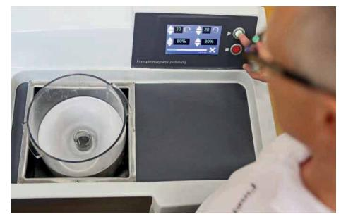
The Finespin polishing and deburring range is available in four models, the F28, F35, F45 and F50. Powered with a single phase 240 V supply, the compact machines have a maximum component capacity of 1, 3, 5 and 8 kg respectively. The smallest F28 model has a 280 mm by 280 mm work table, while the largest F50 can support parts up to 600 mm by 540 mm.
