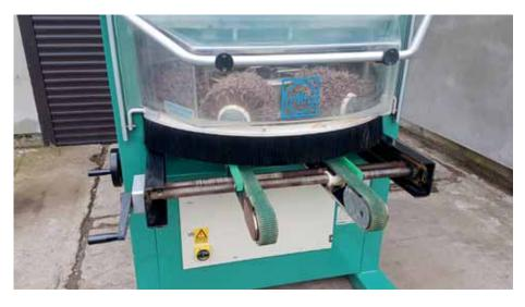
developed and the first automatic feedthrough machine for denibbing of, for example, kitchen cabinet doors was presented at the LIGNA exhibition in Germany:
