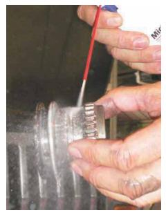
Here the operator cleans a similar gear to excellent results using an HFC-based formulation with a much safer toxicity rating
