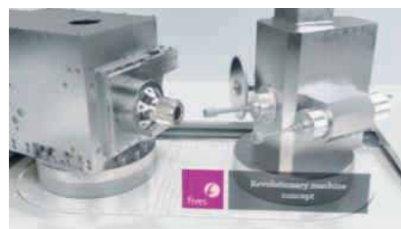
Twin Turret machine axes (two rotary, one linear)
