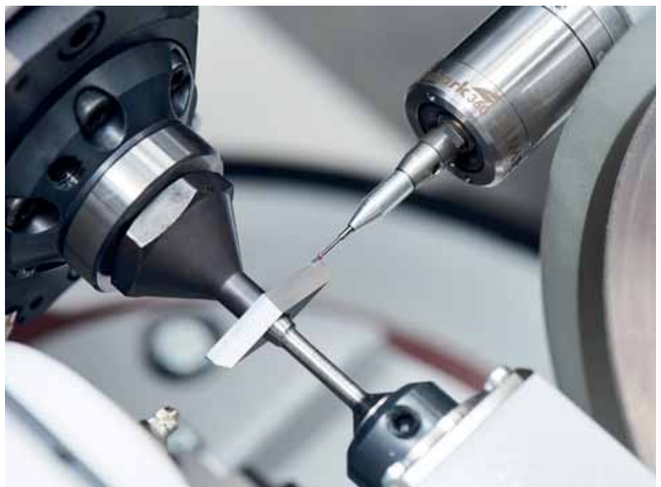
Agathon's 3D measuring probe gives the user complete freedom to measure specific features of a workpiece in the workspace
