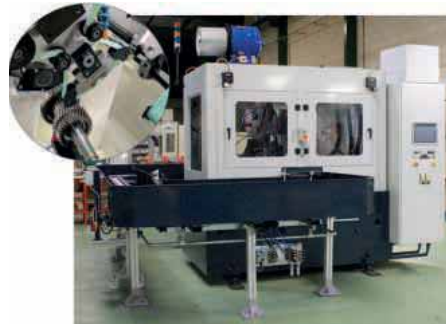
A CMA machine using formed superfinishing shoes and equipped with recirculating horizontal workpiece load/unload conveyor for production of gearbox shafts
