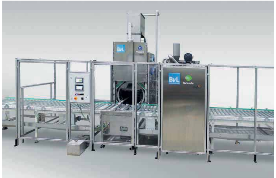
The NiagaraDFS basket washing system from BvL with the Nevada external vacuum dryer allows a very wide range of gearbox parts to be reliably cleaned in short cycle times
