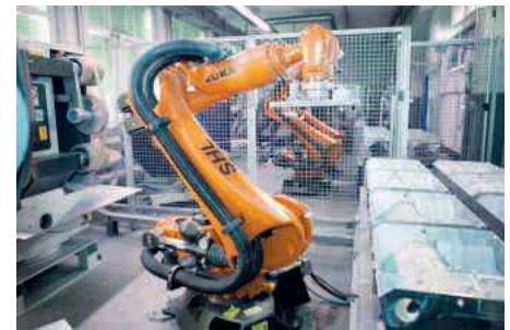
KR 120 R2500 pro robots grind and polish aluminum housings
