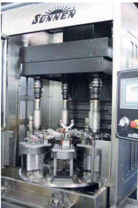
The 4-spindle VSS-2 honing system used by Cloyes Gear to hone the bores of VVT stators. The segmented bore of the powder metal parts is finished to a roundness of 50 microns and total tolerance of 80 microns
