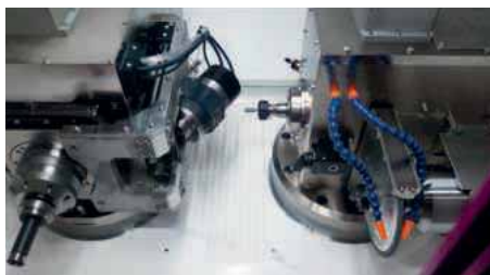
TTG350 shown here configured with in-situ dressing spindle, I/D grinding, O/D grinding, turning and metrology
