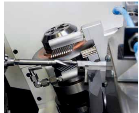
Junker coolant nozzle tracking - the automatic coolant nozzle tracking and clever measurement system with automatic dimensional correction are ideal for unmanned production
