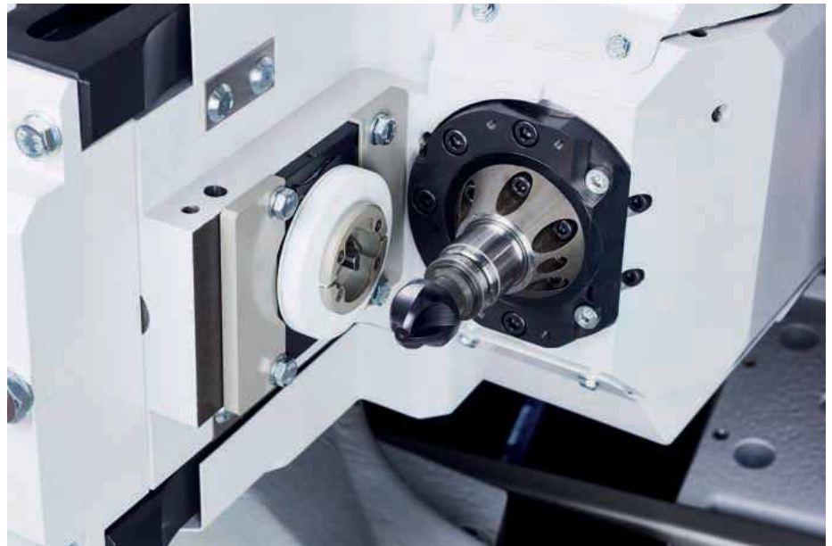
The clamping system HSK forms a universal interface on the machine side on which a wide variety of workpieces can be mounted
