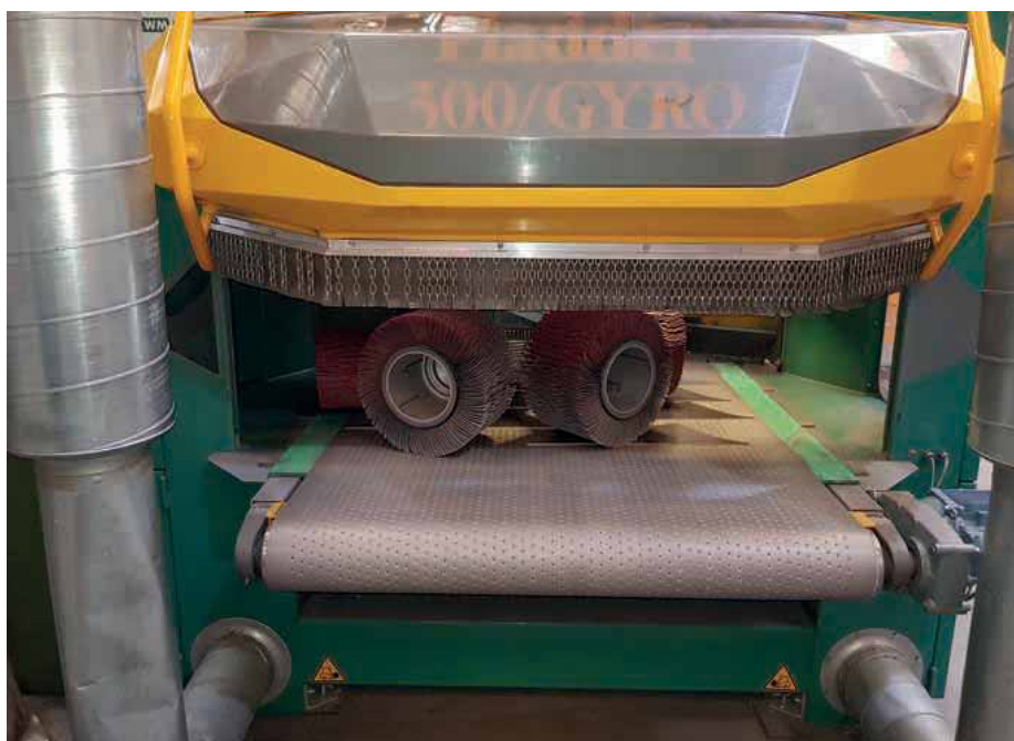
KWM Weisshaar uses the deburring roller 400 x 250 x 200mm from boeck on the FLADDER deburring machine, thus saving 50 percent of the machining time
