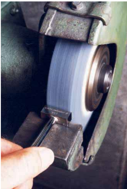
A VH1 Diamond Multi-Point Hand Dresser shown dressing a grinding wheel on a tool and cutter grinder
