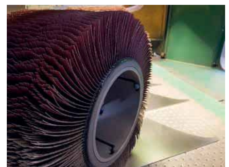
Despite the higher abrasive fabric content, boeck's deburring rollers are very light. This reduces the bearing loads in the machine
