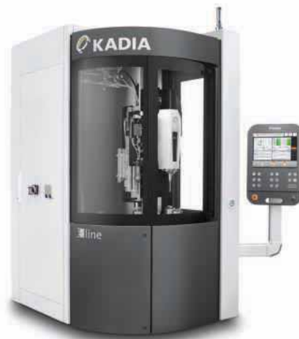
E line Eco honing machine with the HMC100. KADIA now supplies every honing machine with the high-end controller
