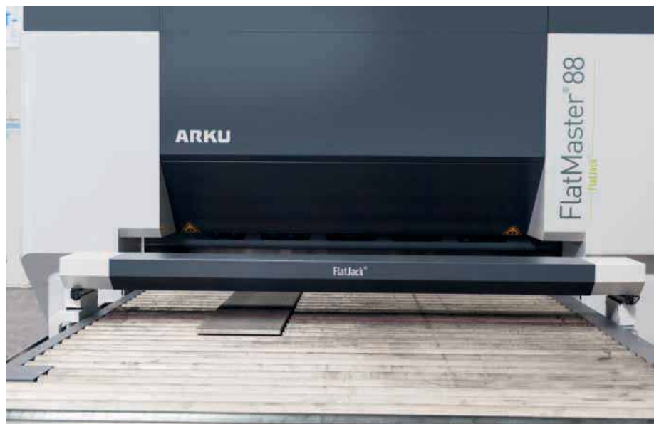
The FlatJack flatness control system measures the leveled parts with a precision in the tenths of a centimetre range
