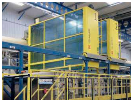
Two overhead transporters dip flight bars carrying aluminium components into 15 tanks sequentially. Up to five jobs can be processed simultaneously in the line
