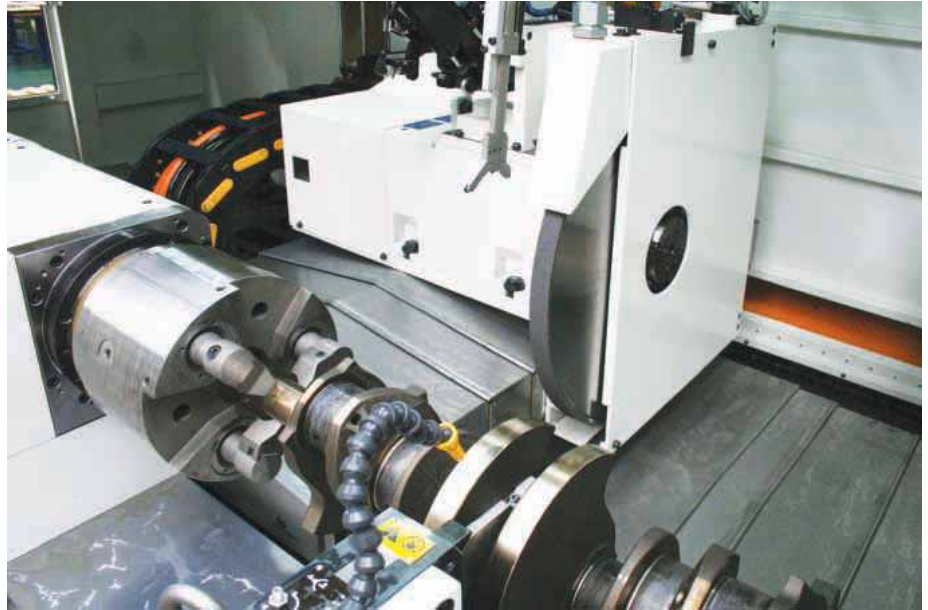
Workhead with pressurised electrospindle, hydraulic self-centring with three self-compensating jaws chuck system and self-centring hydraulic automatic steady rests
