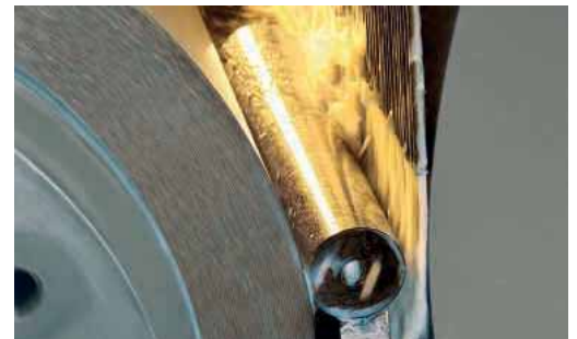
With the JUPITER 200 S, centreless grinding can be carried out on a huge range of workpieces, from pipes to hydraulic pushers
