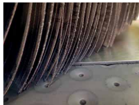
The individual abrasive cloth flaps are cut in a contactless manner via lasers. This results in no grain losses in the abrasive fabric
