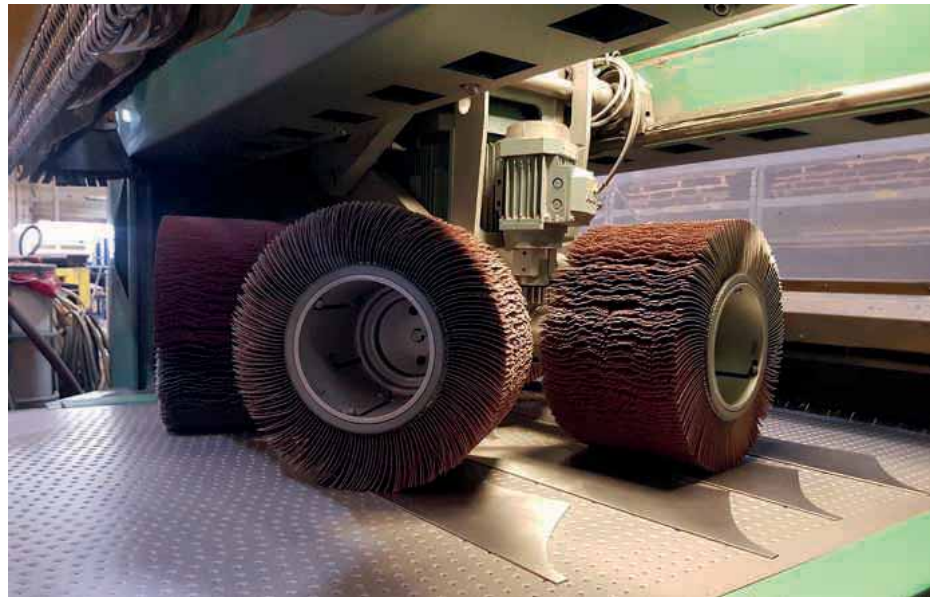
Due to the arrangement of the flaps in the grinding or deburring direction, KWM achieves an improved level of edge rounding than with the tools previously used
