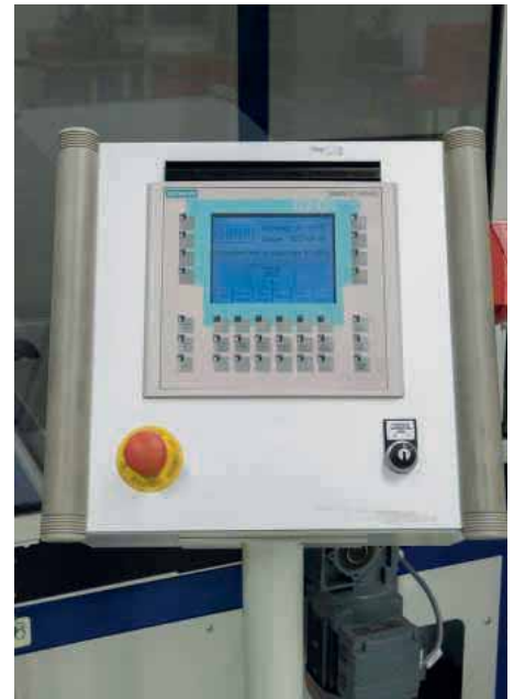
Different cleaning programmes are stored in the controller of the solvent cleaning machine. Process parameters are visualised
