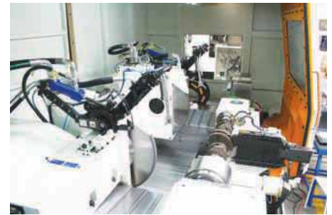
The design of the machine is characterised by the overlapped and crossed arrangement of the main Z longitudinal and transversal X machining axes
