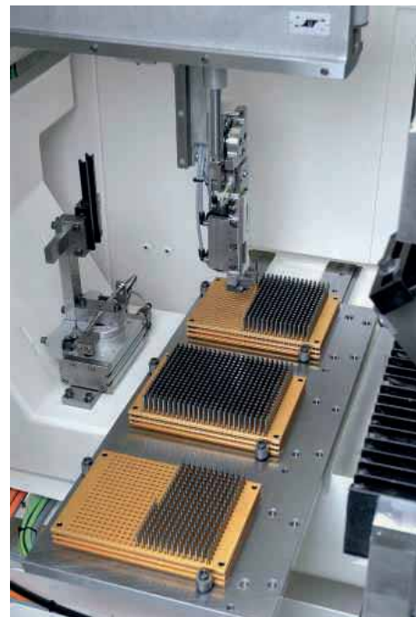
The automatic loading device also facilitates unattended operation
