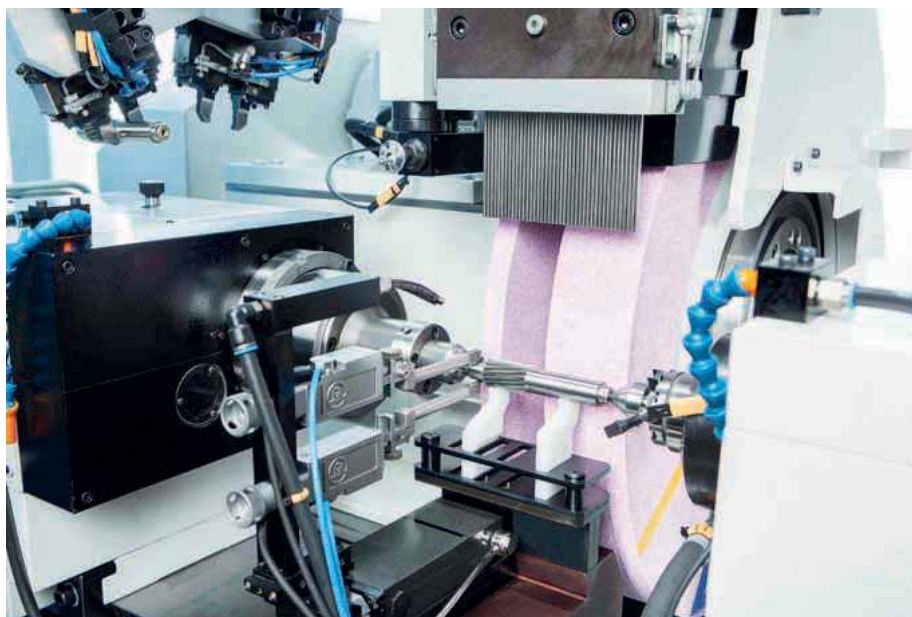
Together with the Jucrank 6S CBN high-speed grinding machine, the Numerika machines crankshafts. Here the journal is being ground
