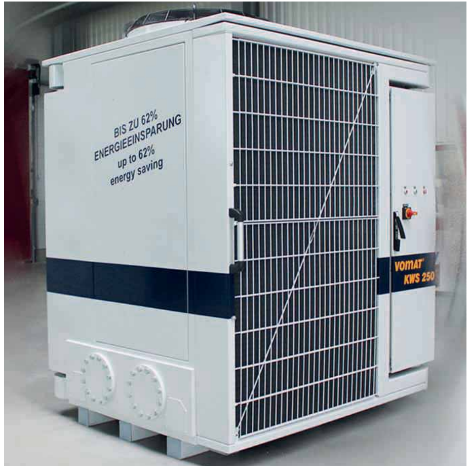
New is the energy-saving KWS 250 chiller with integrated circulation pump and compact Eaton controls. It has a cooling capacity of 250 kW for brine operation. The control accuracy is +/-1.0 K
