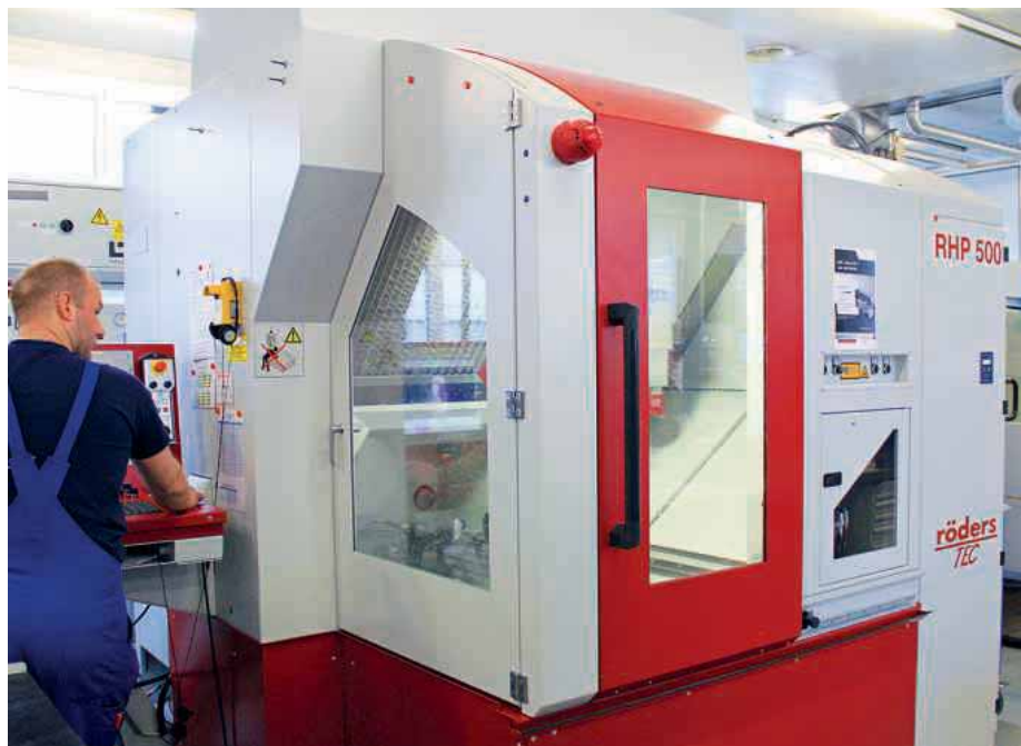
The Rödgers RHP 500 machining centre installed in the Feintool shop proves itself for HSC milling as well as for jig grinding jobs involving ultra-hard materials with up to 66 HRC
