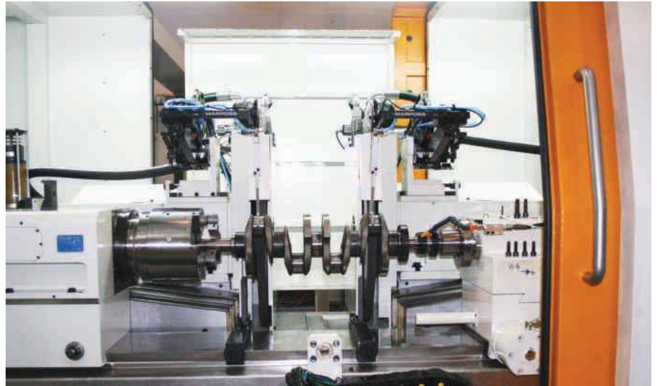
The new DU grinding machine can be configured with one wheelhead or two wheelheads side by side
