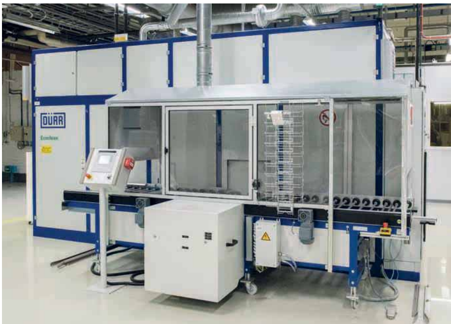
For quick and reliable degreasing of the cemented carbide and cermet indexable inserts, ranging from 5 to 50 mm in size, the hydrocarbon-based cleaning system comprises two flood tanks with separate filter circuits, and an extra 10 cm has been added to the length of its work chamber
