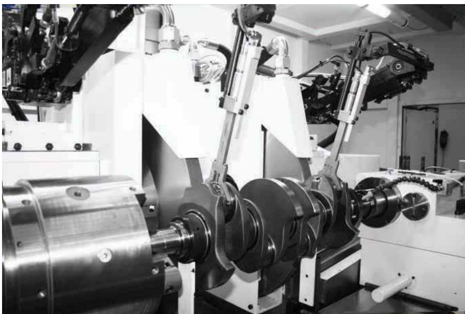
Eccentric grinding of the crankshaft takes place by orbital tracking of the crank pin. An in-process measuring system with a fork follows and continuously measures the orbital movement of the pin during grinding
