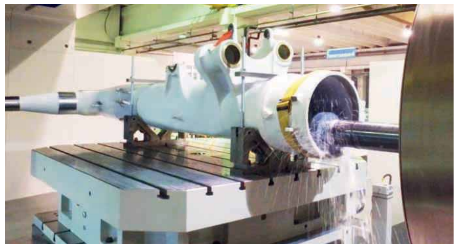
Above & below: In a single grinding machine, the orbital grinding of external and internal diameters is performed without moving the workpiece
