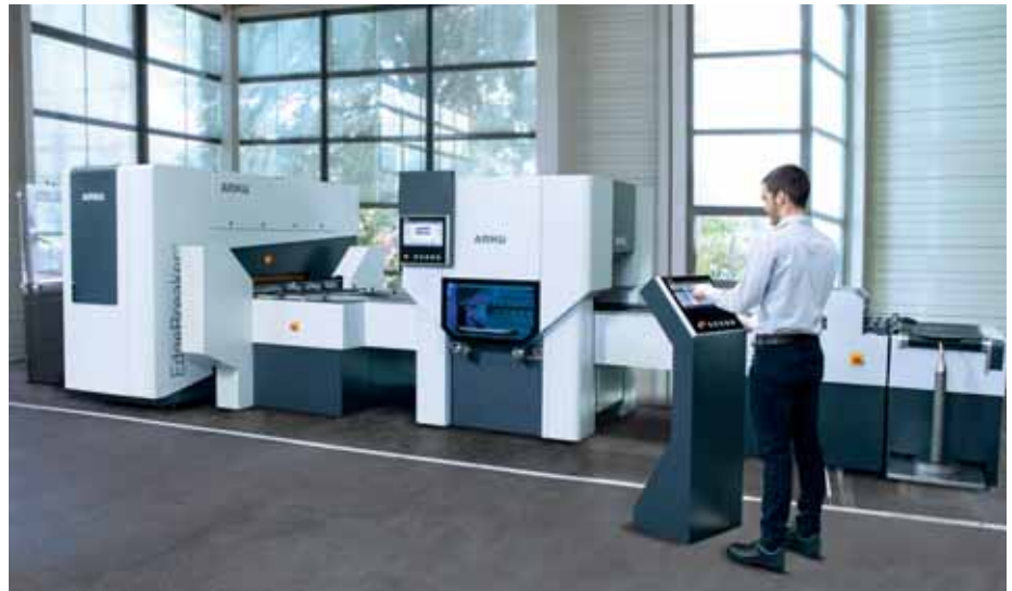
Levelling, deburring, flatness testing: the production line presented at the EuroBLECH covered multiple production steps
