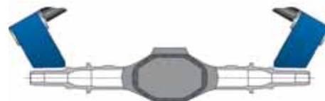
Axle shafts - the two grinding spindles on the Numerika reduce the total cycle time by more than half
