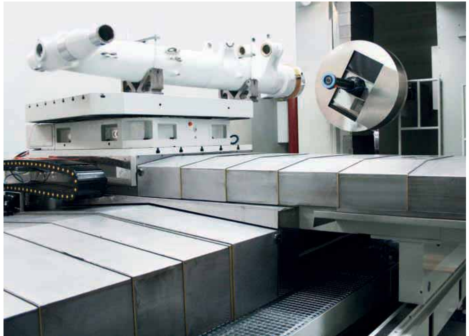
The rotary table is moved by the overlapped and crossed arrangement of the main machining axes, Z and X, which allows ample operating capacity with reduced dimensions on the ground
