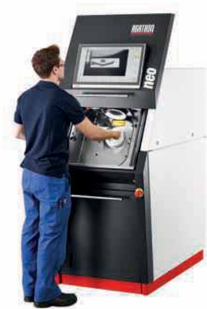
The PCD tips were pre-processed on the Agathon Neo laser processing machine
