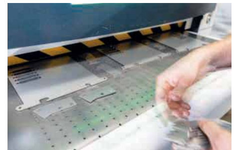
The vacuum table allows small parts to be processed automatically
