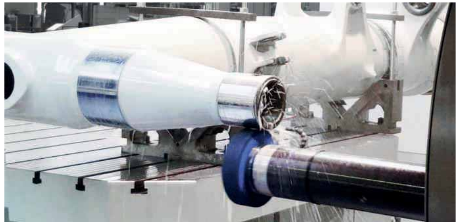
Above & below: In a single grinding machine, the orbital grinding of external and internal diameters is performed without moving the workpiece
