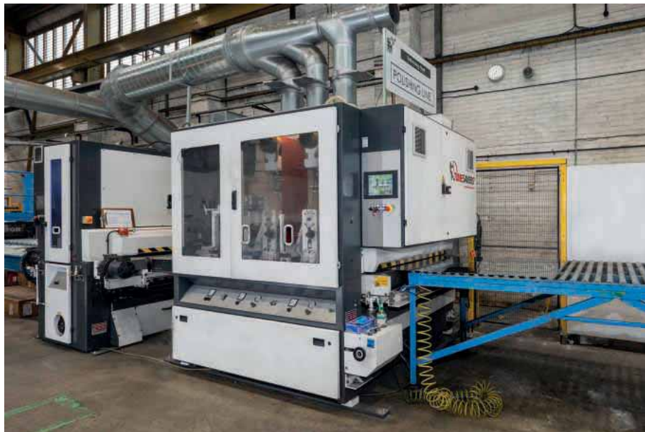
Top, middle and below: The Timesavers 72-1600-HL Hairline finishing machine installed at Rimex. Combined in a flowline with a Timesavers 62-1600-WWB (belt+belt+brush) finishing machine
