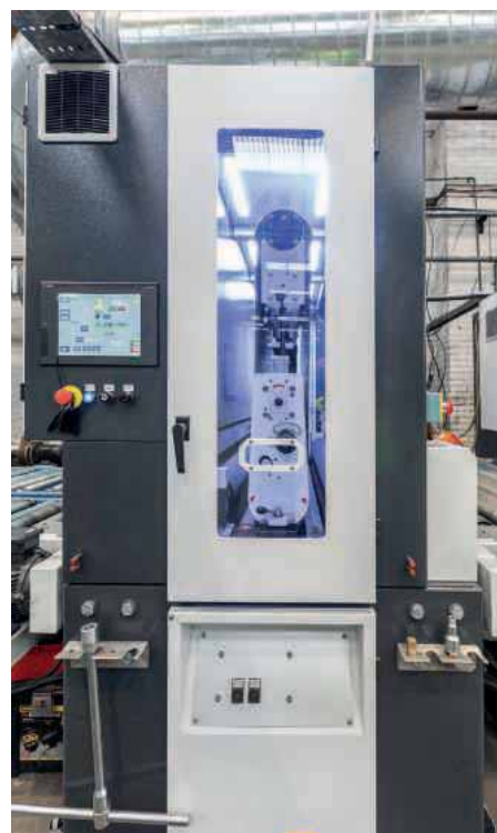
Top, middle and below: The Timesavers 72-1600-HL Hairline finishing machine installed at Rimex. Combined in a flowline with a Timesavers 62-1600-WWB (belt+belt+brush) finishing machine
