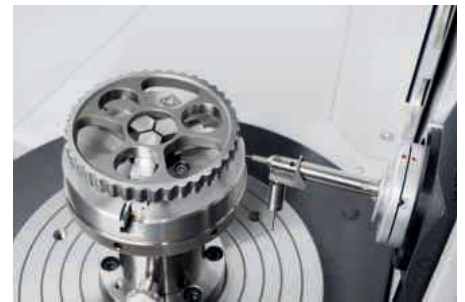
Cycloid measurement on a Klingelnberg precision measuring centre
