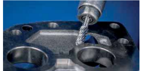
30 percent higher stock removal rate for steel than conventional TC burrs with cross cut - ALLROUND from PFERD
