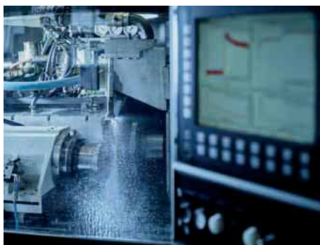
ToolScope analyses the machine data gathered during grinding and displays it as a diagram on the machine control panel. Photo: TYROLIT
