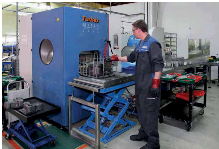
A basket of pinions entering the Turbex Java process chamber at the automotive transmissions manufacturer
