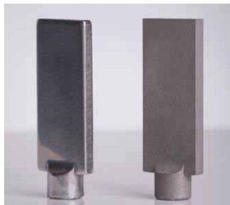
Stainless steel test bar before and after surface finishing by Fintek and LJMU (who also conducted mechanical testing) of simple test bars additively manufactured by CAM
