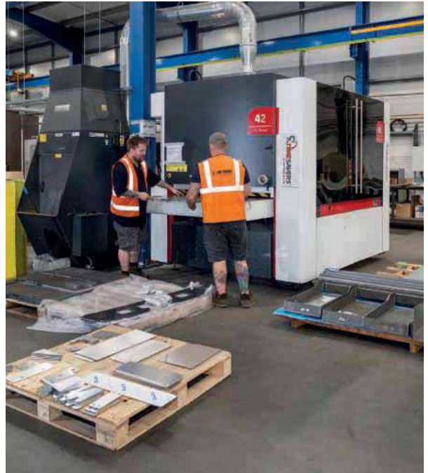
The Timesavers 42 Series RB machine from Ellesco installed at Optima Metal Services is easing a deburring bottleneck and generating new business
