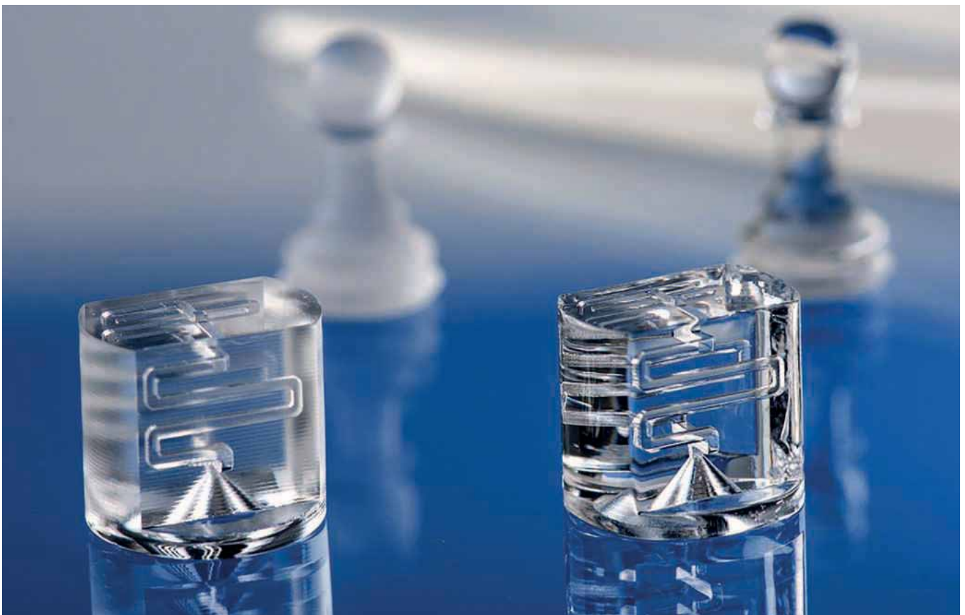
Microfluidics made of fused silica ( 5 \times 5 \times 7 \text{ mm}^3 ) manufactured by SLE (left) and laser-polished (right)
