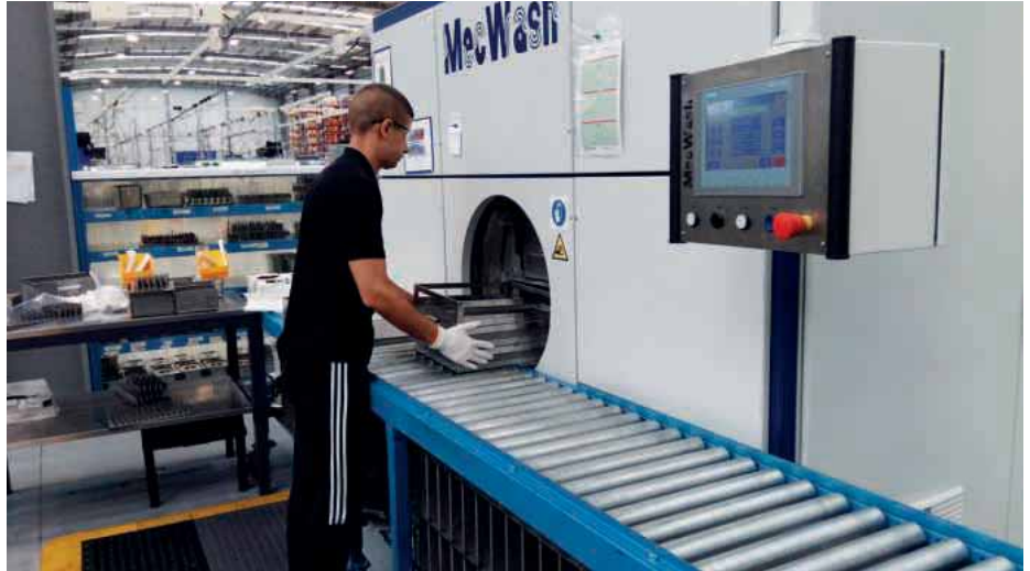
The new facility allows achieving very high cleanliness requirements for a wide range of parts quickly and efficiently. A major contribution here makes the ultrasound equipment (photo from MecWash Systems Ltd)
