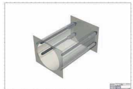
Two Sonopush Mono HD rod transducers with 25 kHz (1,500 watts) and 40 kHz (1,200 watts) each were integrated into the working chamber (photo from Weber Ultrasonics)
