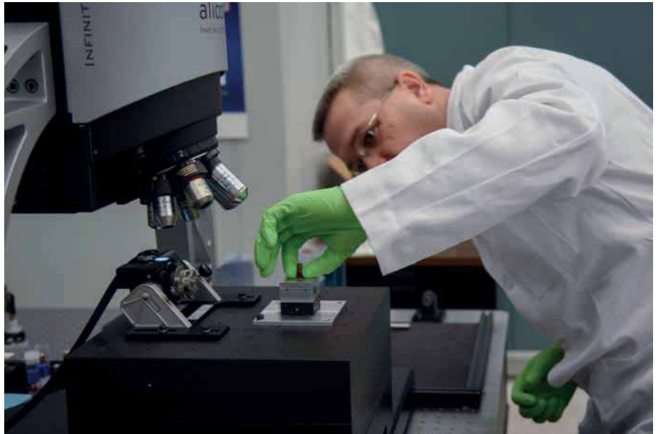
NIST physical scientist Mike Stocker places the bullet, wrapped in a silicone sleeve, on the microscope for a new run
