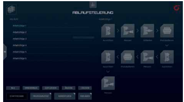
Photo 2: The sequential control allows for a straight-forward compilation of workflows
