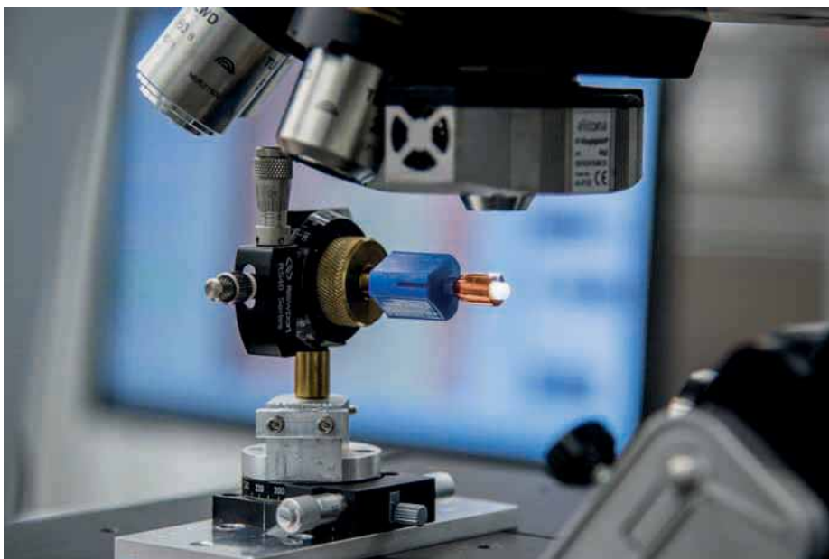
Prior to each scanning run, the system is calibrated using a known sample: NIST Standard Reference Material 2460, better known as the standard bullet
