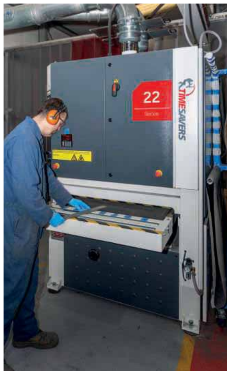
The variable table height allows thin sheet and thicker plate to be processed
