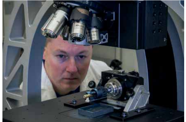
Thomas Brian Renegar examines the positioning of the bullet before the scanning run begins.
