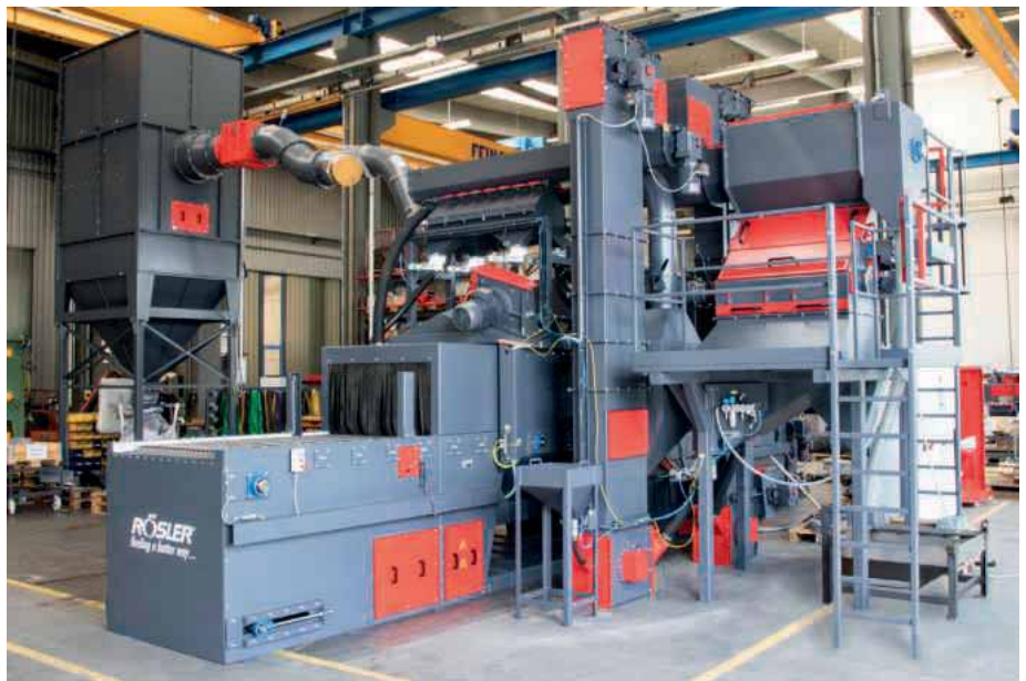
With numerous accessories, like a high-performance magnetic separator, the wire mesh belt machine RDGE 1250-4-F was perfectly adapted to the tough operating conditions prevailing in foundries
