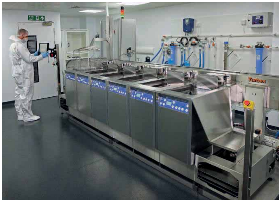
Aimed at precision cleaning applications, the Turbex automated ProLine 2 550 aqueous system has three wet stages and a dryer plus load and unload station
