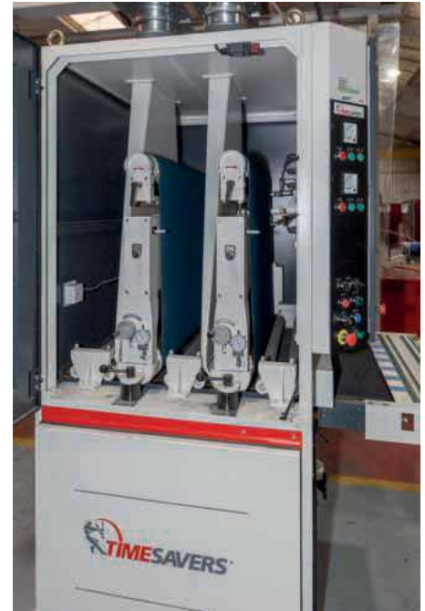
The twin-head configuration improves productivity
