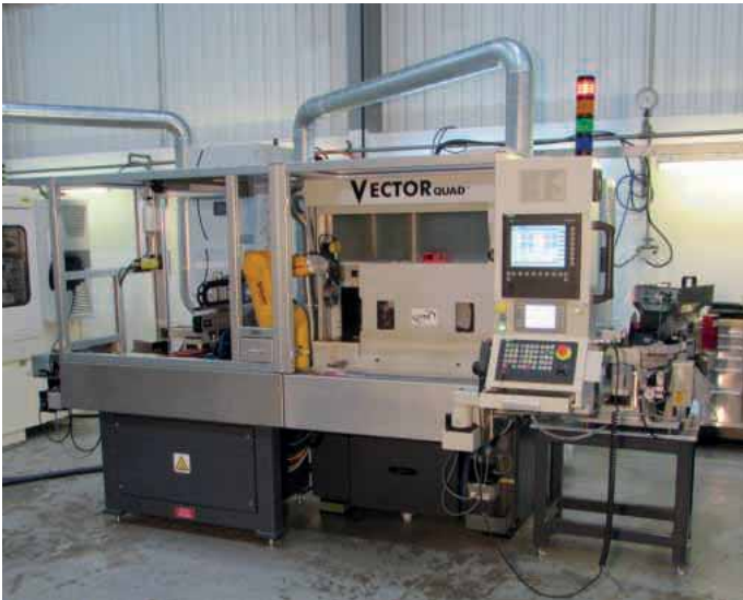
The Vector Quad Cell giving optimised autonomous production for peel grinding carbide tool blanks
