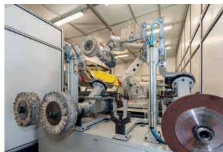
Left & right: Automations engineer Musa Banaddawa manually positioning the robot (for illustration purposes), and the four position polishing mop station
