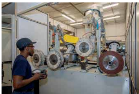
Left & right: Automations engineer Musa Banaddawa manually positioning the robot (for illustration purposes), and the four position polishing mop station
