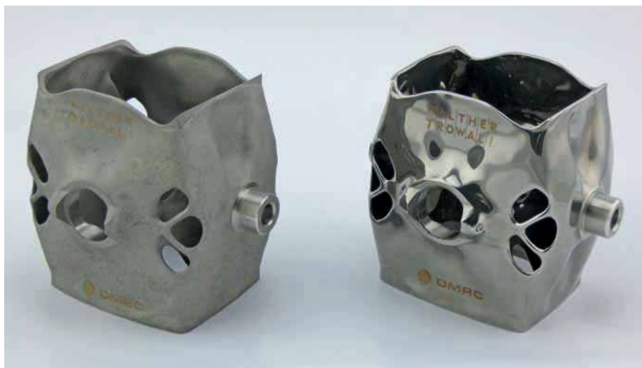
A 3D printed gimble frame before (left) and after the "trowalizing" process
