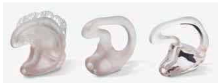
A 3D printed earpiece for a hearing aid before (left), surface smoothing (centre) and after polishing
