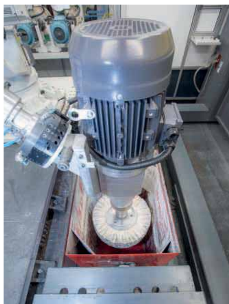
The automated polishing compound station
