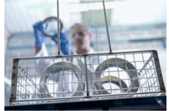
Inspecting metal parts: vapour degreasing cleans and dries parts quickly and effectively
