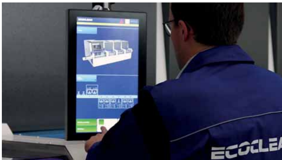
On the 19" flat screen monitor (HMI), all of the system's modules are presented separately and clearly in a complete overview diagram, similar to a smartphone display
