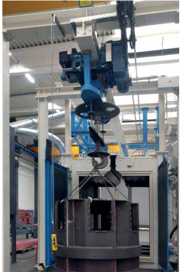
The transport system of the shot blast machine can handle castings weighing up to seven metric tonnes
