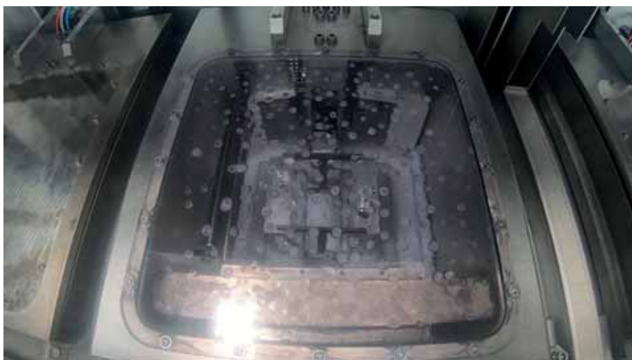
The workpieces are also cleaned and dried as single parts. For these processes injection flood washing, spray cleaning and selective rinsing as well as high-velocity air blow-off and/or vacuum drying are available
