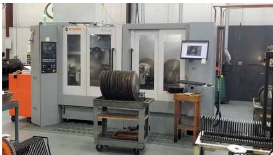
The VOLLMER CHX 840 + HS circular saw grinder for machining the tooth faces and tooth tops in a single clamping operation
