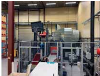
While one batch of work pieces is processed in the rotary vibrator, a second batch is passing through the separation station and, in case of wet processing, through the dryer
