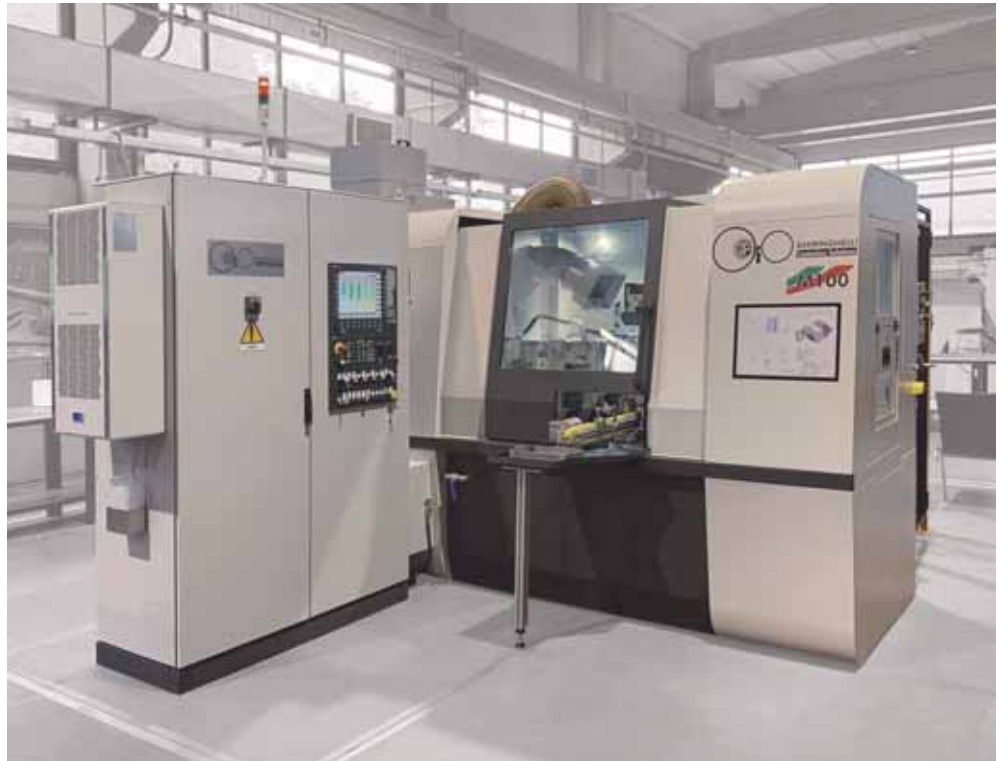
The Ghiringhelli M100CNC6A is a centerless grinder with 6 NC axes suitable for the grinding of components with O.D. from 0,5 to 20 mm
