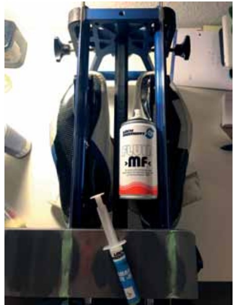
A clamped skate during lapping operation with LACH DIAMANT paste 3 µm and spray can Fluid »MF« to reactivate dried up paste
