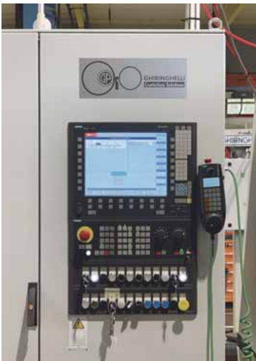
The Siemens 840D SL NC unit includes the exclusive Ghiringhelli HMI
