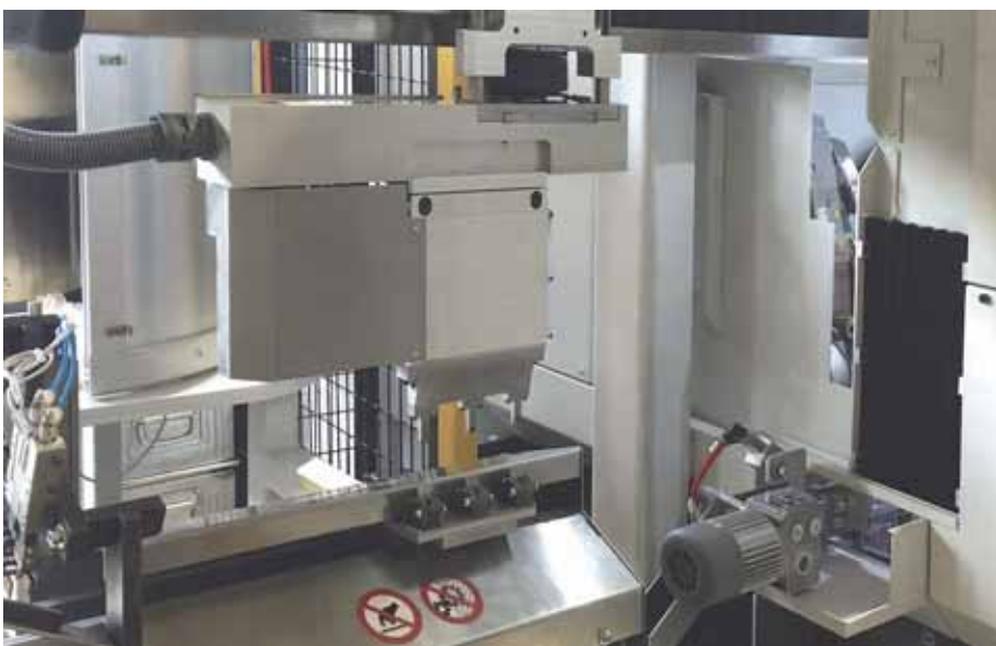
All centerless grinding machines can be equipped with different customized types of automatic feeding and loading systems
