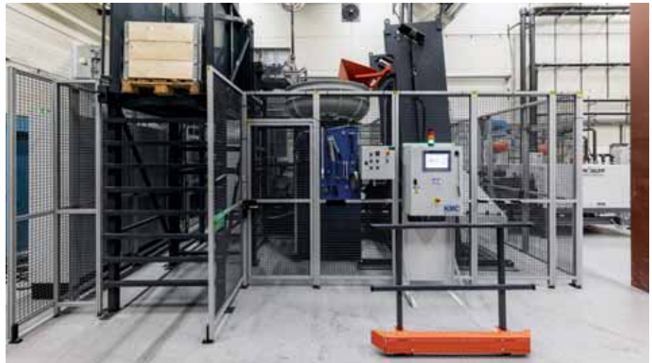
The package, consisting of a rotary vibrator, a hot air belt dryer and a semi-automatic centrifuge, allows the parallel processing of two workpiece batches in either dry or wet model
