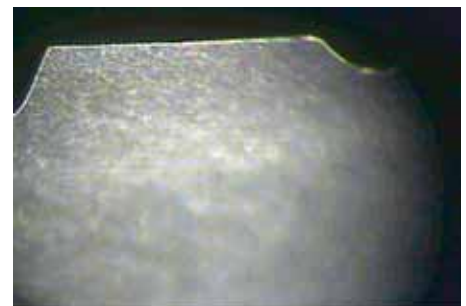
Cutting tool edge after processing on the MF machine
