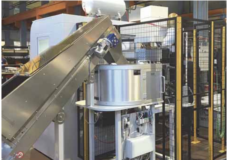
Detail of the feeding system composed of hopper bowl feeder, orientation and positioning unit of the components
