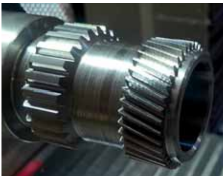
A hobbed helical gear and a skived straight gear on the same shaft
