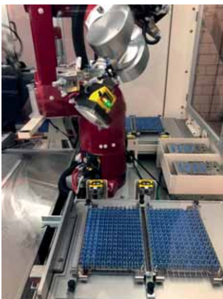
Mass deburring of parts for the automotive sector
