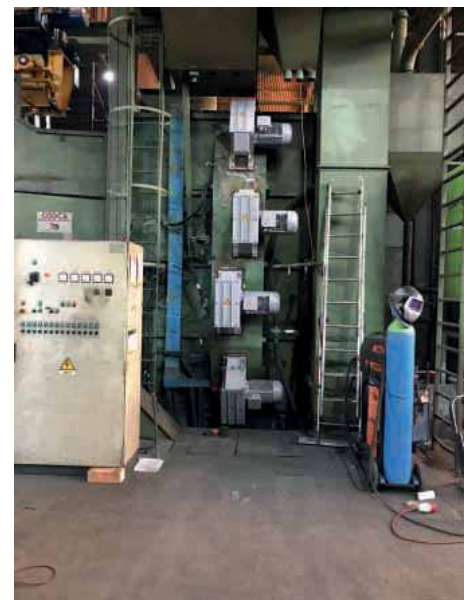
Three new AGTOS high-performance turbines on the modernised overhead conveyor blasting machine
