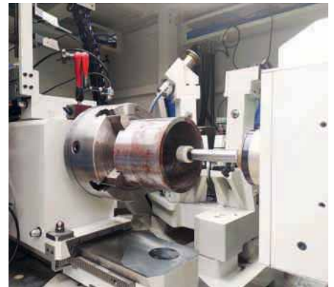
The headstock with C-axis is placed on a U-axis swivel table. Behind the headstock, special stands positioned at 45^{\circ} is arranged on a rigid support for dressing of the wheels
