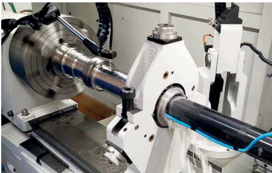
The GSB line allows it to be configured for high precision grinding of very deep holes
