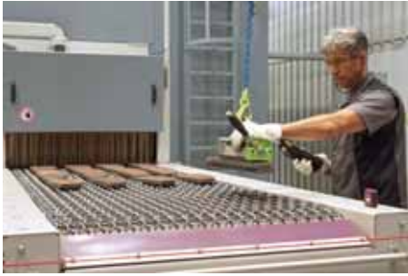
Loading the AGTOS Type BS wire mesh conveyor shot blast machine
