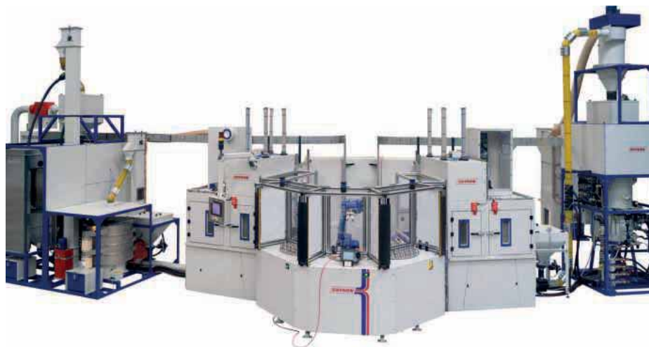
Large automated, robot loaded, twin blast machines, for shot peening turbomachinery turbine blades or medical implants
