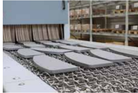
AGTOS wire mesh conveyor shot blast machine outlet
