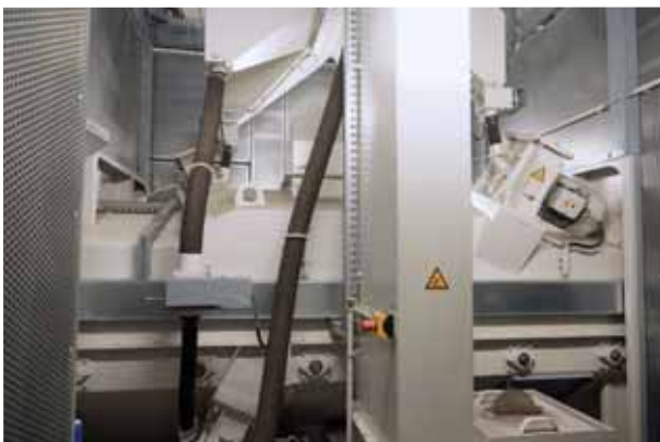
Behind the acoustic insulation: the blasting chamber is at the heart of the wire mesh conveyor shot blast machine
