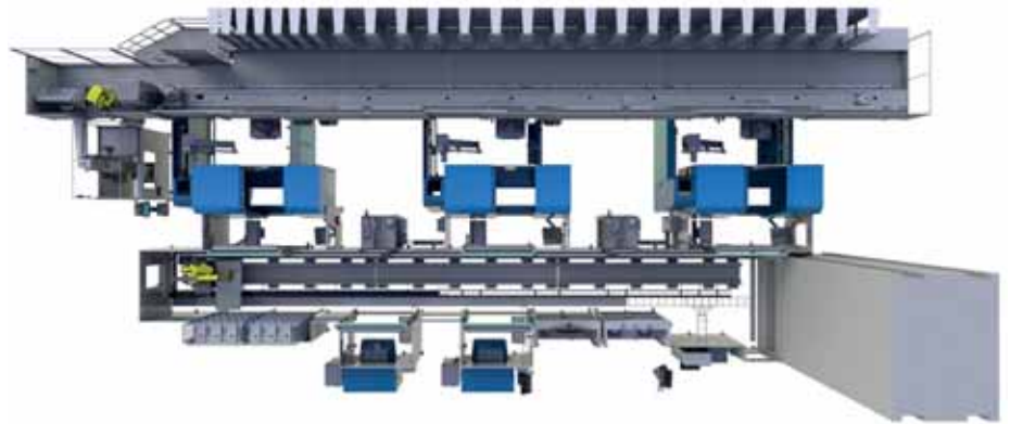
The system from a birds-eye view: grinding machines are in the middle with tool gantry storage on the above and robot with it's rail below
